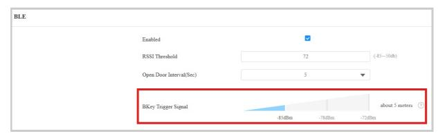
• **Bkey Trigger Signal**: Three ranges are available, setting door opening distance to about 5 meters, 3 meters, and 1 meter.
